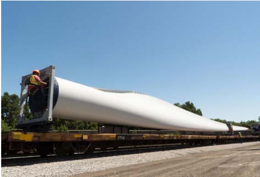
Wind blades are nearly as large as a football field and require over three rail cars to safely transport them.
